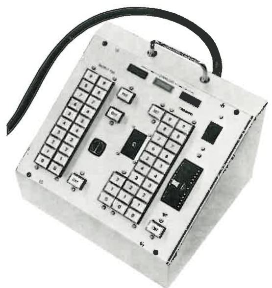
Figure 4 Portable control unit. Attached to a flexible cable, this enables all the principal control functions to be carried out from a convenient position on the studio floor.
