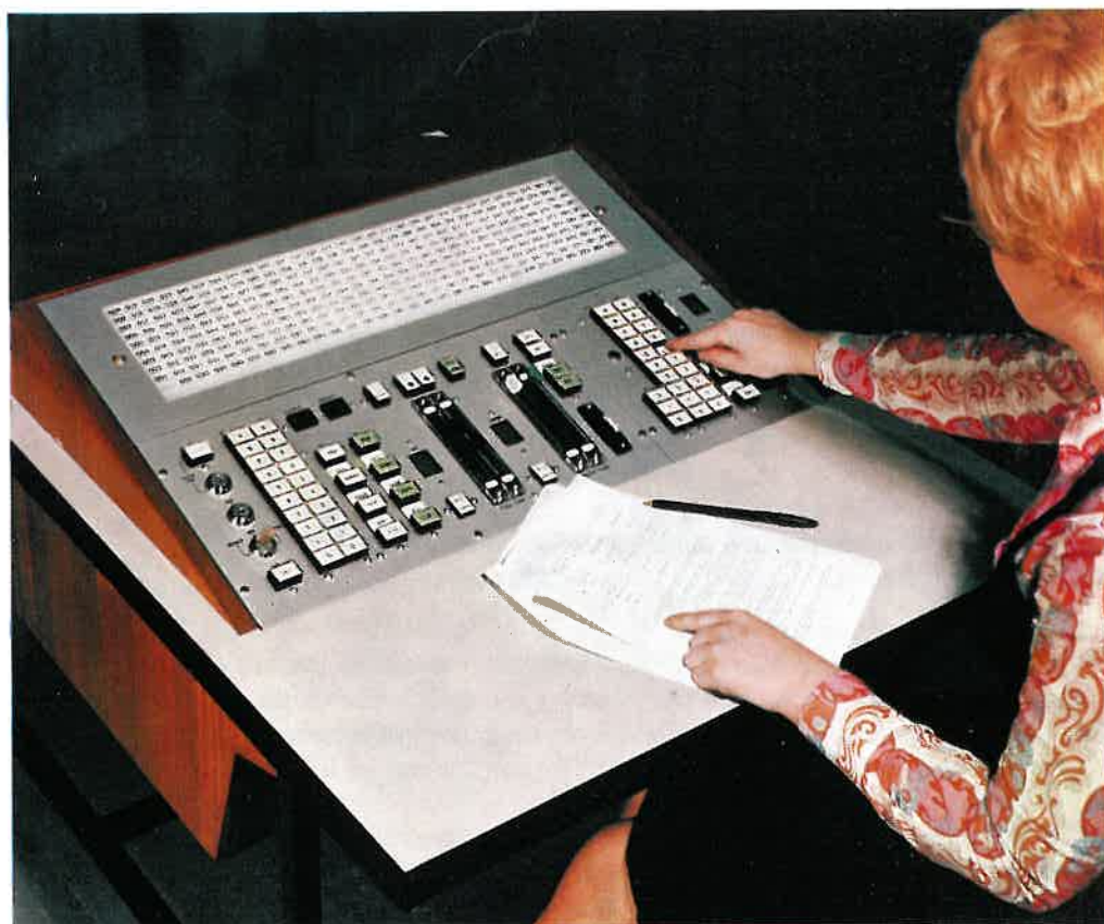
Typical Q-File control desk suitable for a 300 dimmer installation.
